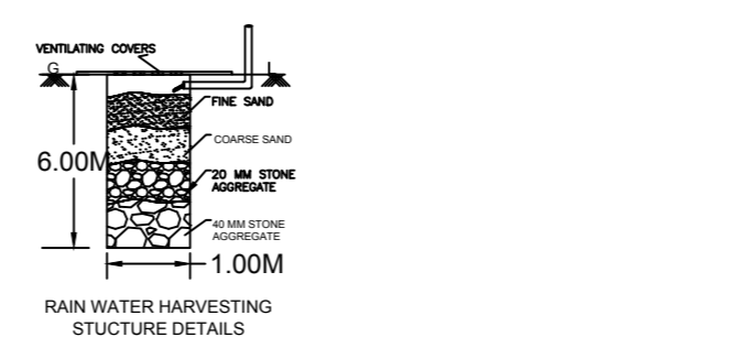
RAIN WATER HARVESTING STRUCTURE DETAILS
